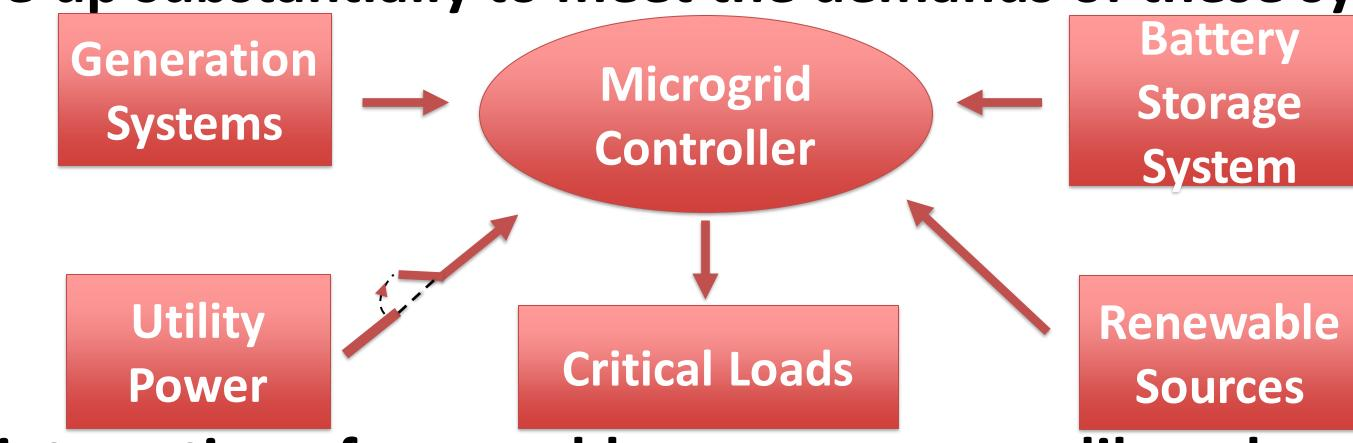
The idea behind a microgrid is to have a back up system in place separate from a primary grid so outages are minimized in disruptive events. Resilience is increased since the inclusion of a subsystem limits the risks
